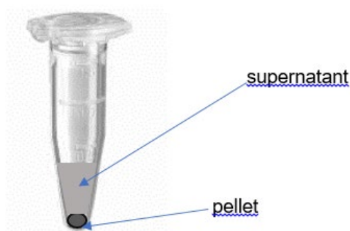
Figure 5. Pellet and supernatant after centrifugation
