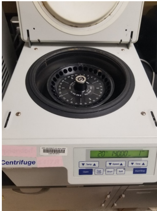
Figure 4. Microcentrifuge with rotor with space for 1.5-2.0 ml microcentrifuge tubes
