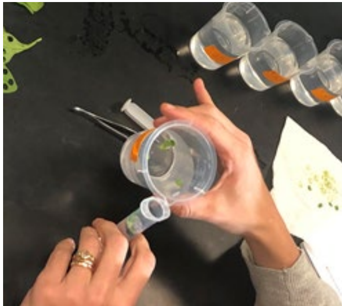
Figure 2. Removing air from the spinach leaves
